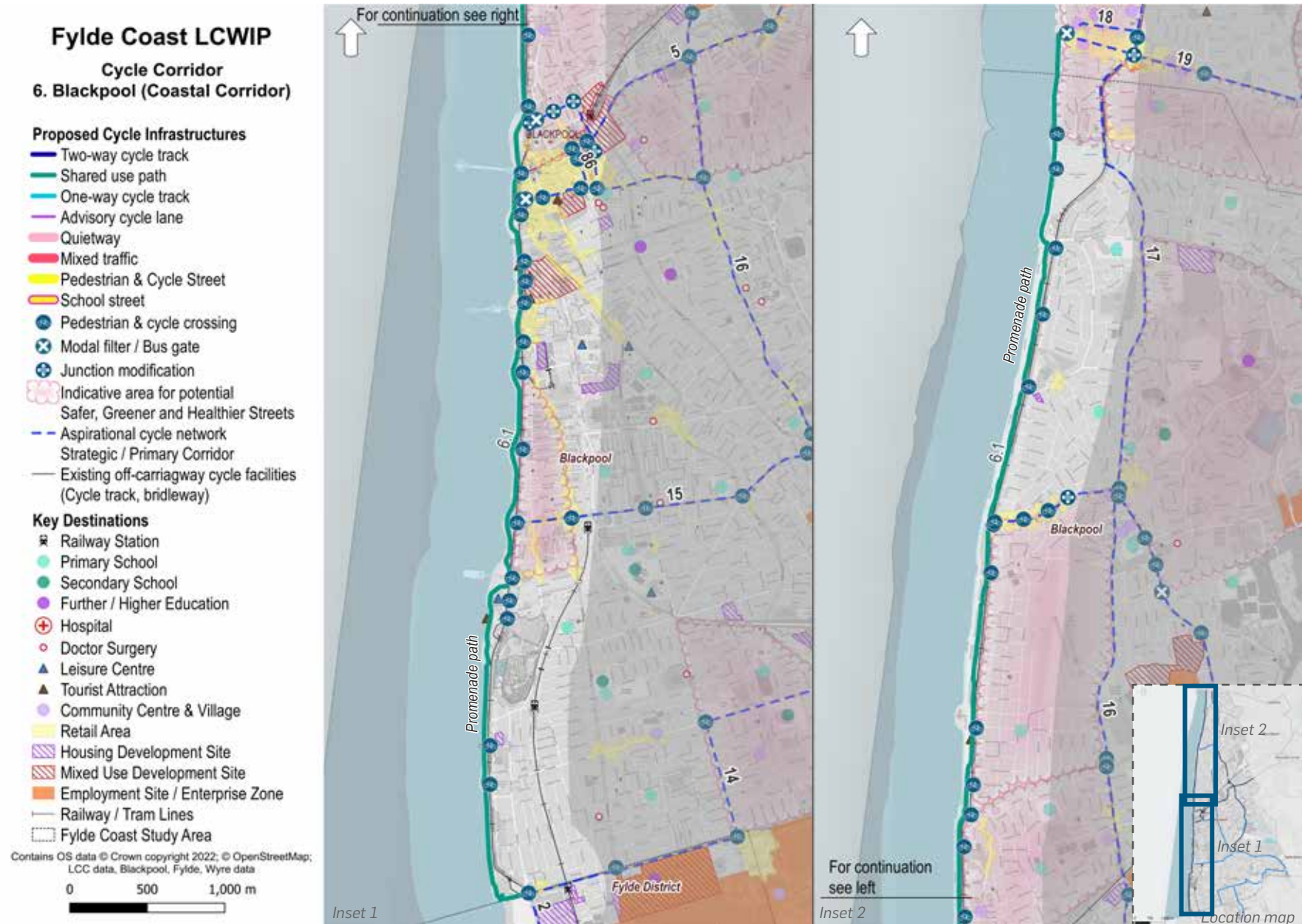
Figure 64. Indicative proposed cycle infrastructure, Cycle Corridor 6: Blackpool (Coastal Corridor)
